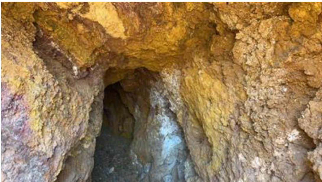
Photo 3: Oxidised carbonate replacement mineralisation in exploratory adit 80m south of previously reported high-grade lead and zinc values. Sample 24RR-AL16: 3.2% zinc
